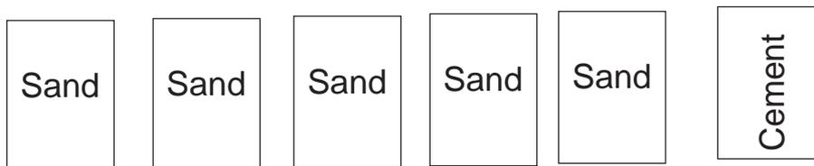
Mortar is made by mixing 5 parts by weight of sand with 1 part by weight of cement.
