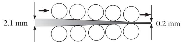
If the percentage reduction is constant on each pair of workrolls, find that reduction. Also, if the incoming speed is  $1 \text{ m s}^{-1}$ , what is the outgoing speed?
