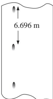
Returning to the first problem in which there are five pairs of workrolls with an input thickness of 2.1 mm and output thickness of 0.2 mm, a mark is noticed on the finished strip.
